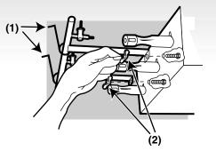
5) Slide the burner assembly out from under the guide screw and washer(1) in the corners of the cooking box.
